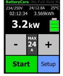
No Full Charging can be switched on via Setup menu, while BatteryCare is enabled. This function is preventing your battery to be fully charged. Once finalising (constant voltage) phase is detected, car charge stops. For your information status "No Full" stays orange until reset with Start button.
