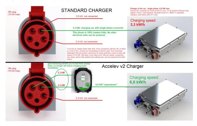
Typical 16A charger connected to 16A x 3 phase home grid (10 kW max capability, standard in Europe), drains one phase totally. Charging speed is about 3,3 - 3,5 kW. Nothing else can be connected to that phase (breaker will turn off the power). Also, no 3-phase tool can be used while charging an EV car.
