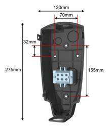
3. Attach the bracket using fasteners that are appropriate for the type of wall material, drilling pilot holes if necessary. Use the supplied screws only if mounting the bracket directly to a wooden stud. If mounting to another type of wall (hollow, masonry, etc.), use fasteners that are long enough to securely anchor the Wall Connector and can hold at least 36 kg.
