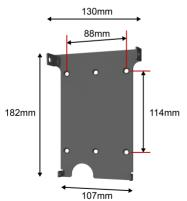
Position the bracket so that the Wall Connector is located at a maximum of 150 cm from floor level. The minimum height is 45 cm if mounting indoors, and 122 cm if mounting outdoors.
