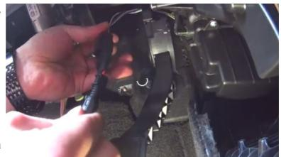
screwdriver to open TeslaChip, programmer is an orange one. TeslaChip can be left at cabin silencer that is installed in all Tesla cars under steering wheel, or you can put it in any place, tightening it to the surface with included zip ties.
